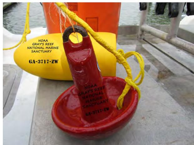
Gray's Reef vessel operators use an 8 pound mushroom anchor attached to a line and buoy float to mark the location of divers underwater. (Photo: Todd Recicar, Amy Rath)
